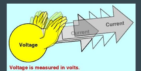
The higher the energy (voltage) of each charged particle, the greater the potential difference or ability of electrons to move their way through a circuit.
