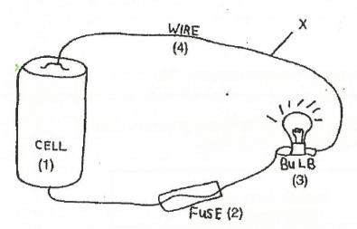
5. The top of the cell in the diagram represents the positive terminal. Trace the flow of electrons through the four items in the circuit, starting from point X in the diagram. Indicate the proper order by placing the numbers of the components from left to right in the spaces below.
