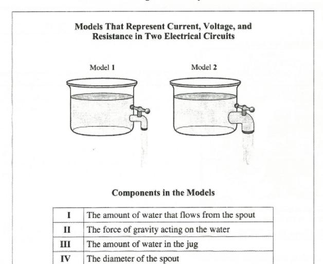
3. Which of the components in the models represents resistance in a DC circuit?
